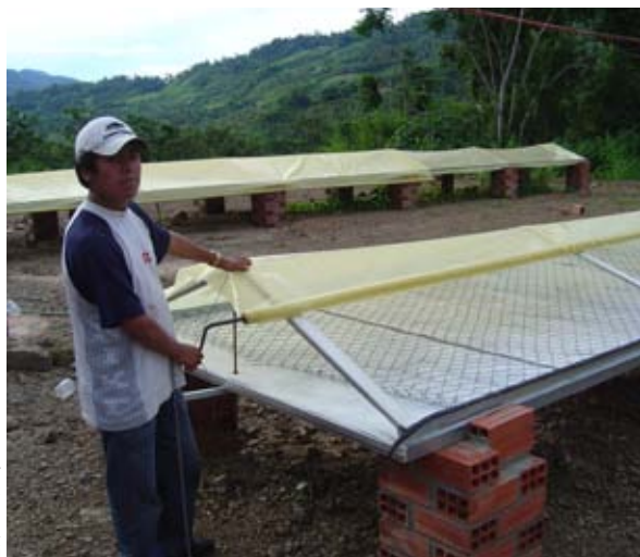
Panel for aromatic herb drying in Caranavi
